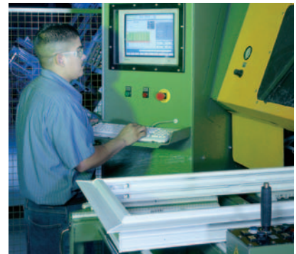
After welding, we remove the excess material with precision equipment for an aesthetically superior finish.
